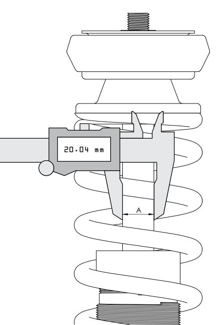
To ensure you receive the correct Coiloverlift kit for your coilovers, one simple measurements is required. Before you begin, please take a few moments to make sure the shock rod is clean, ensuring an accurate result. We strongly suggest using a caliper to take these measurements. A digital caliper is recommended, however, a cheap \$5 analog caliper will do in a pinch.
